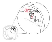
Release the front cover latch: According to the body pattern, 1. Pull down the latch and do not release it; 2. Turn the toggle button to the right to lock the latch, and the front cover can be opened directly without the need for an iron rod.
