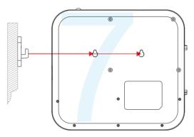
The hanging hole on the back of the device can be hooked on the hook
